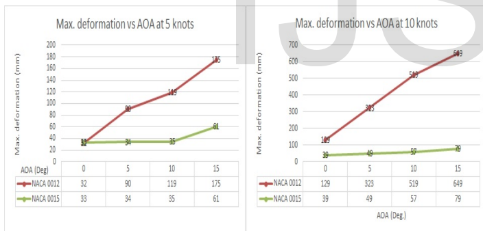
Fig.10. Comparison of deformation at 5 and 10 knots towing speed
